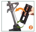
2. Separate the metal quad rails (covers) into 2 pieces, the Top Cover (3 rails) and the Bottom Cover (1 rail). Install the Top Cover onto the barrel by aligning the inner two spinal cords against the central groove area on the Barrel Nut, and push for a tight fit.
