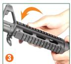
3. Press downward the Top Cover to pull back Delta Ring, and then release toward the barrel to allow the Front Handguard Cap to fit snugly inside the front rim of the Top Cover. Make sure that the Top Cover is well situated.
