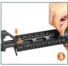
5. Tighten all four screws using the provided Allen wrench to secure the top and bottom covers. The Quad-rail is ready for most versatile accessory applications.
