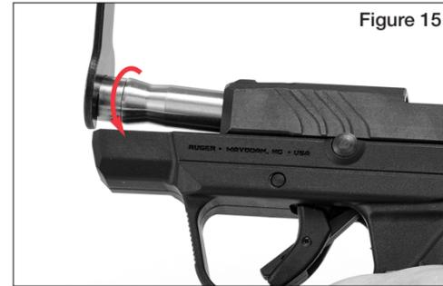
**NOTE:** Do not use a cheater bar on the supplied thread adapter/cap wrench as damage can occur to either the thread adapter, cap or barrel.
