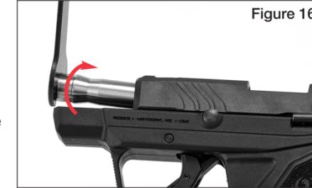
3. Install the thread adapter by carefully screwing it **counterclockwise** onto the threaded portion of the barrel by hand.
