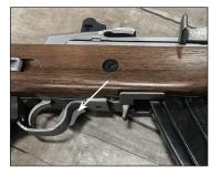
Remove the magazine by pushing and holding the magazine latch forward while drawing the magazine forward and downward.
