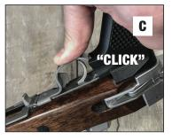
Cycle the slide handle and safety a few times to be certain the components are correctly assembled. Put the safety back "ON." Reinsert an empty magazine and fully withdraw slide. The bolt should lock open automatically.
